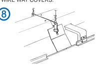
AFTER JOINING FIXTURE SECTIONS, IN-STALL COUPLER STRAPS AS SHOWN ON EACH SIDE OF FIXTURE. JOIN USING ALIGNER CLIPS (SUPPLIED).
