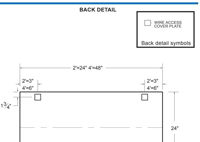
NOTE All fixtures must be installed, wired and grounded in accordance with the National Electric Code and all other applicable codes.
